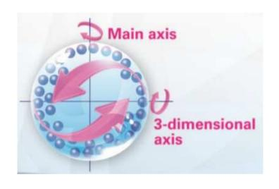
The sample pulverized by the Brazil nut effect goes to the bottom.
