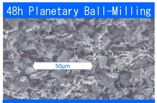
Sharp edge and bulky shape of the particle by strong impact force.
